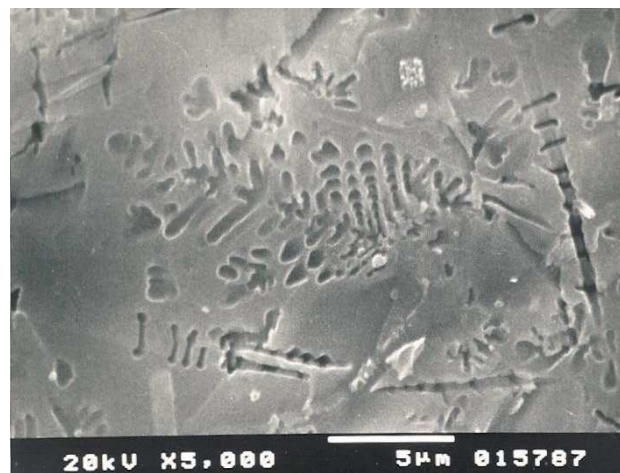
Figure 2: SEM micrograph of well-shaped dendritic \text{AlPO}_4 crystals
