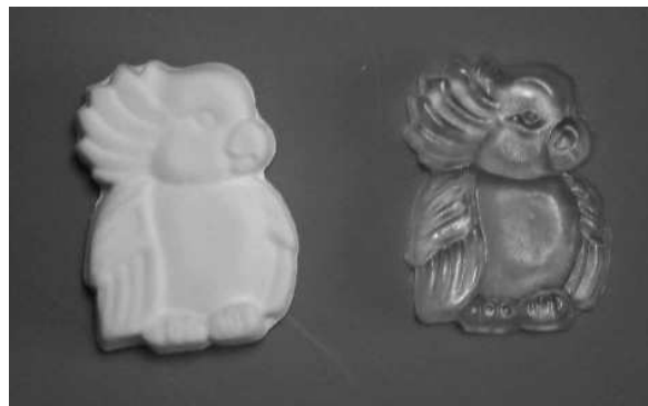
Fig. 7 Parrots with reduced shrinkage. Green body (left) and sintered glass (right)
