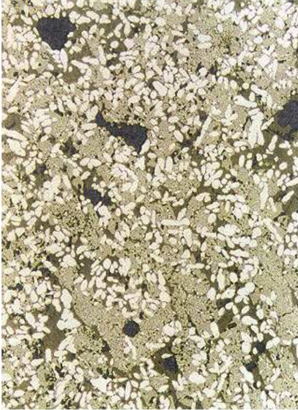
Figure 3: Typical microstructure of a fused cast AZS 41 material- Monofrax CS 5
