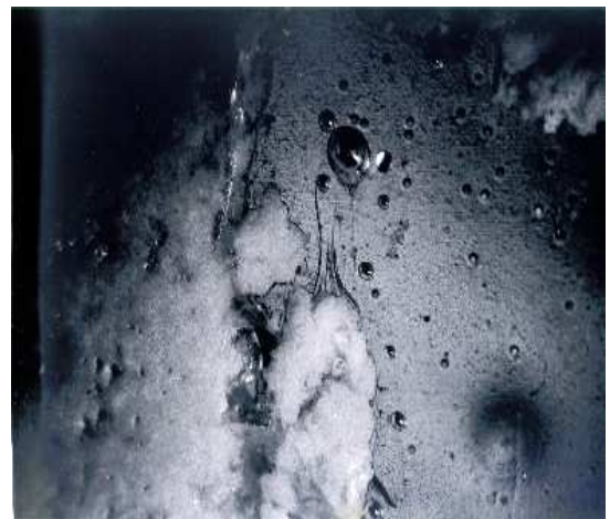
Figure 6: Polished section of boundary layer region between an AZS block (left) and a glass melt (right), with bubbles and knot glass rising from art the part of the \text{ZrO}_2 seam.
