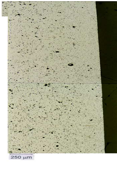
Figure 7: Boundary layer area of an isostatic pressed CR95WA block (left-96 % \text{Cr}_2\text{O}_3 , 4 % \text{TiO}_2 ) with a soda-lime silicate glass (right) after a reaction time of 120 hours at 1.450 °C.
