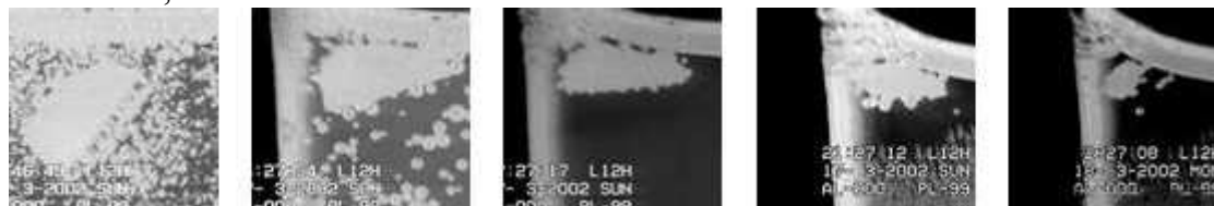
Fig. 1 Decrease of size of a porcelain particle at 1300 °, t_{\text{fig. 1-5}} = 0, 1, 4, 8, 13 h
