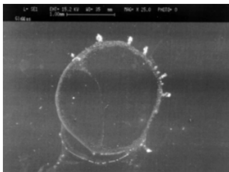
Figure 7. SEM micrograph showing stain formation on glass surface.
