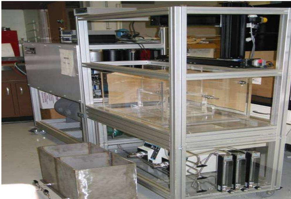
Figure 1 – Physical modeling (glycerin tank to simulate glass flows) [photo from GTI, D. Rue]
