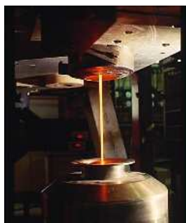
Figure 1. Pouring a glass melt in an industrial facility
