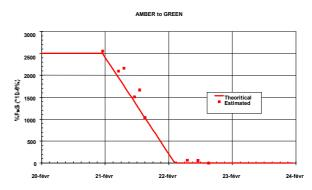
The operation has to be conducted in a minimum of time while preserving glass quality. The challenge is to switch from the old color range in scheduled time to the new target with a minimum of time. This involves an appropriate boosting of the coloration or discoloration. The operation must be carried out carefully and must be neither too slowly or too fast in order to avoid stopping before reaching the target or going through it.
