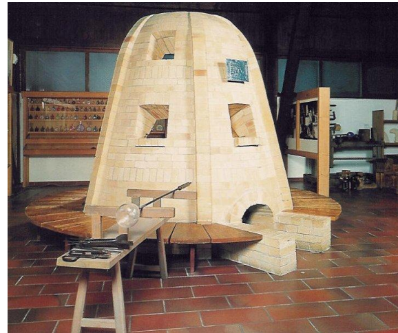
Glass melting furnace according to Agricola
